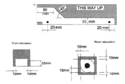
One END of the block has a pre-drilled hole (~ 18 mm diameter) to accommodate the rocket motor (not supplied – to be inserted and ignited on the day of the race by the Race Officials). This end of the block will be the rear of the car. (Marked "Rear elevation" on the diagram.)
